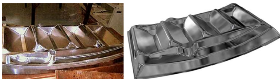
Fig. 8 The original design, a 23-piece weldment in comparison with the proposed one-piece design
